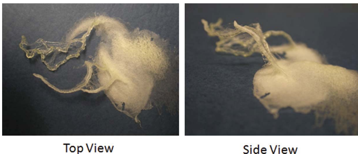
Figure 6 Effect on mat from PPFcPM-BAPO collecting in same area on target (scale bar is 20 and 2 \mu\text{m} , left to right). [Color figure can be viewed in the online issue, which is available at www.interscience.wiley.com .]
